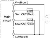
NPN / 1 switch output and 1 analog output
