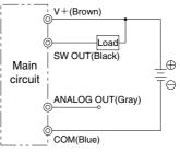
PNP / 1 switch output and 1 analog output
