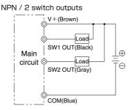
Internal Circuit diagrm and Connection Method
